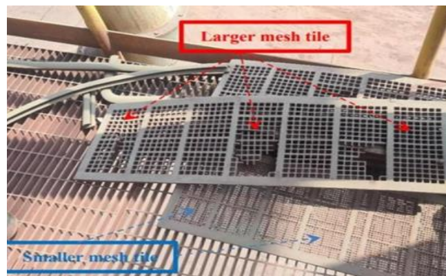
Fig. 4: Larger upper deck polyurethane tile with large aperture and lower deck polyurethane tiles with smaller aperture.
