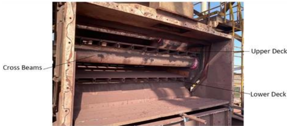
Fig. 3: The screening facility with upper deck holding larger aperture polyurethane tiles and lower deck polyurethane tiles with smaller aperture.
