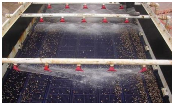
Fig. 5: Wet screening of the iron oxide pellets to remove dust.
