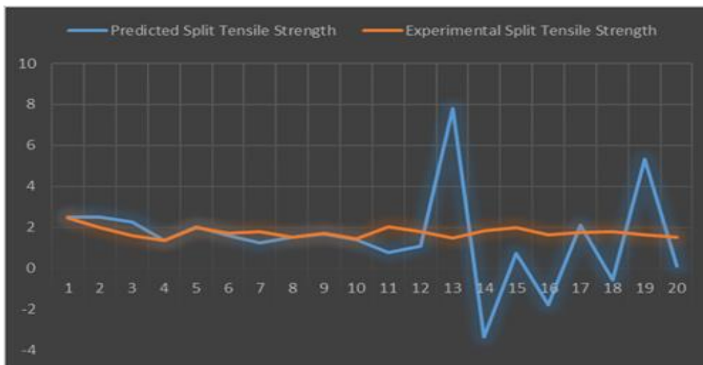
Fig. 4: Comparison of the model predicted tensile strength results against the actual laboratory results.
